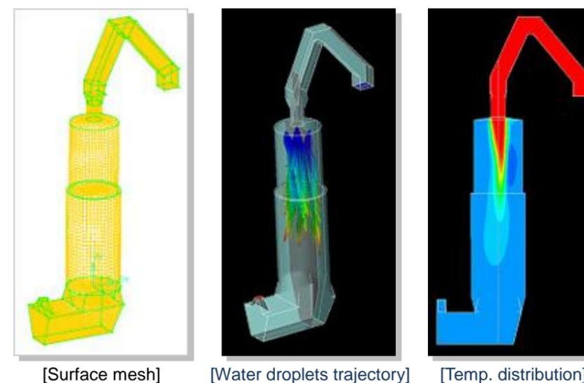
**Example of an improvement on the newly-built gas cooling tower** by simulating the shift of gas flow profile caused by the inlet duct.
